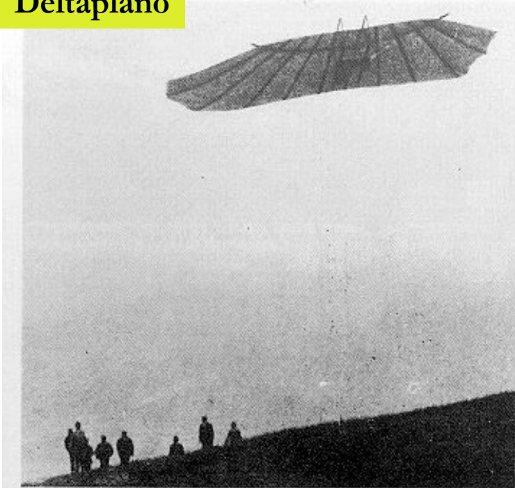
Etrich's 'Zanonia Gleiter' of 1907 was inspired by 'Zanonia Macrocarpa' seeds. It featured one of the main characteristics of most successful flying wings, the wash-out. (H J Nowarra collection)
